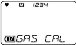
The LCD display shows a battery icon, a signal strength icon, and the number 1234 at the top. Below that, the words "GAS CAL" are displayed in a large font.    | P.43  |
